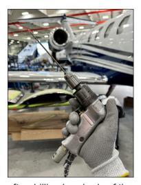
In the mid-2000s, a customer needed a reliable drill for sheetmetal work in aircraft manufacturing and repair. At that time, it was determined that Urvu's UD-50-45 pneumatic pistol drill was the best choice for the application.
