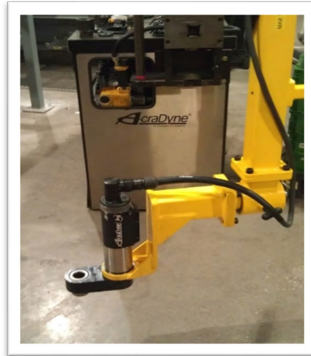
AcraDyne H/T tool w/ offset geared head in torque arm
