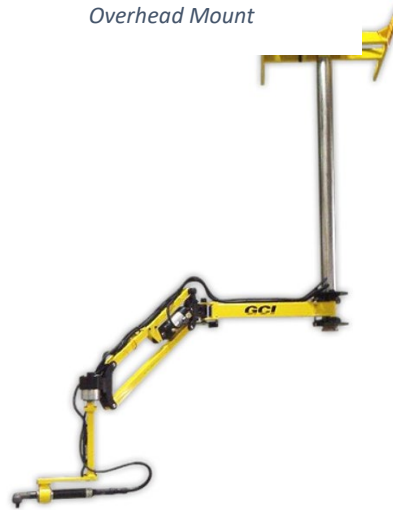
AcraDyne H/T tool w/ offset geared head in torque arm
