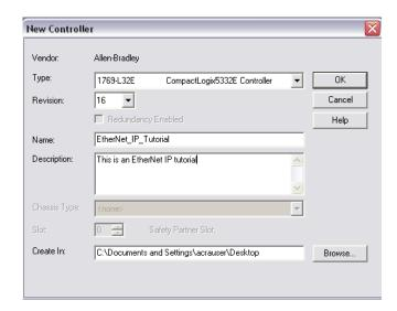
Figure 3. Create a new Project with CompactLogix5332E Controller
