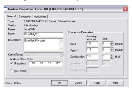
Figure 5 Defining the EtherNet IP Module
