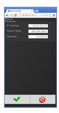
Figure 1 Gen 4 Controller Communication Settings
