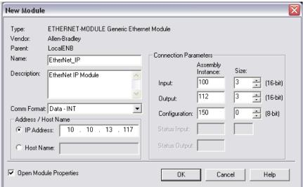
If the AIMCO controller has 3-32 bit input and output integers, RSLogix must have a value of 3 in both the 'Input' and 'Output' field in the 'Module Properties'. It must also have the 'Comm Format' set to 'Data-DINT'. See below.
