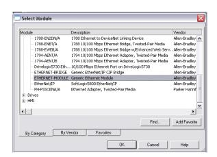
**Figure 4. Define New Generic Ethernet Module**
