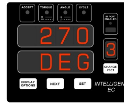
Example: PSET #3, Angle Control Strategy, 270 Degree Target
