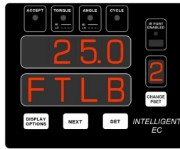
Example: PSET #2, Torque Control Strategy, 25 ft-lb Target
