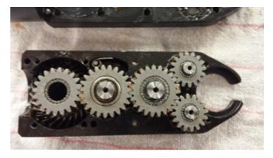
6. Install the output drive gear so that the opening in the upper housing lines up with the opening in the output drive gear. Install the lower housing onto the upper housing making sure that the axle shaft in the lower housing goes into the input drive gear.
