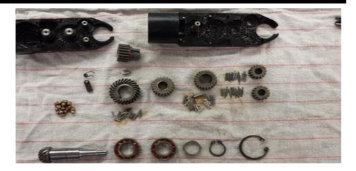
2. Press the two radial bearings onto the crown gear, install the washer and circlip.
