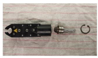
2. Remove the six 2.5mm cap head screws and two 2mm hex flush head from the lower housing, separate the lower and upper housings.
