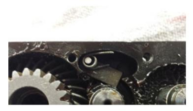
5. Install the key in the input drive gear and install the bevel gear over the key and down towards the gear part of the input drive gear. Install all gears and needle bearings into the upper housing. Rotate the input drive gear counter clock wise until the dog engages with the idler gear.
