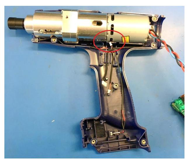
As shown in the picture, the cables of the LED and the motor Hall sensors are mounted in the tooling detail. If the tool has a motor temperature sensor (not shown in the picture), this cable will also be located in this point.
