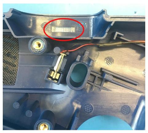
Clip the vibration motor in his position as shown. The rotor of the motor must run free.
