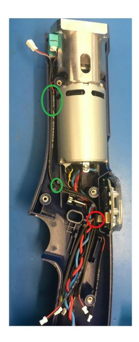
The sensor and LED cables can be positioned in the green marked area. Check that all cables are positioned correctly.
