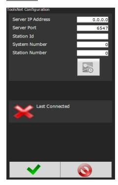
Controller has the ability to send rundown data to a Tools Net server. Once the controller is on the local network, five parameters must be set to store data correctly on the server:
