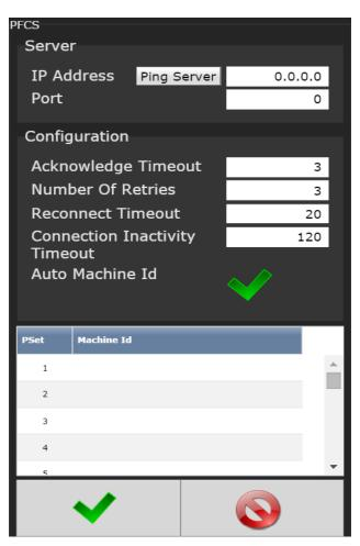
Controller has the ability to communicate over the Chrysler PFCS protocol over Ethernet or one of the serial ports.
