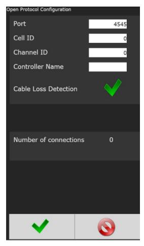
The controller has the ability to accept an "Open" protocol connection. This connection is available over Ethernet and/or the standard serial ports. This connection allows you to enable/disable the tool, set the active parameter set, collect rundown data, and much more.
