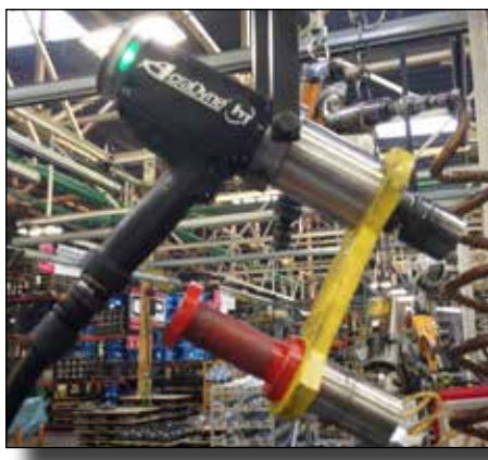
Assembly of Bearing Cap to Carrier
