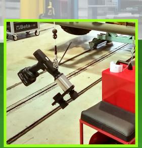
TORQUE RANGE: 185 – 3,688 FT-LB (250 – 5,000 NM) ANVIL: 3/4" – 1" SQ. DR. WEIGHT: 8 – 17.4 LB (9.4 – 18.8 KG) PISTOL & ANGLE CONFIGURATIONS
