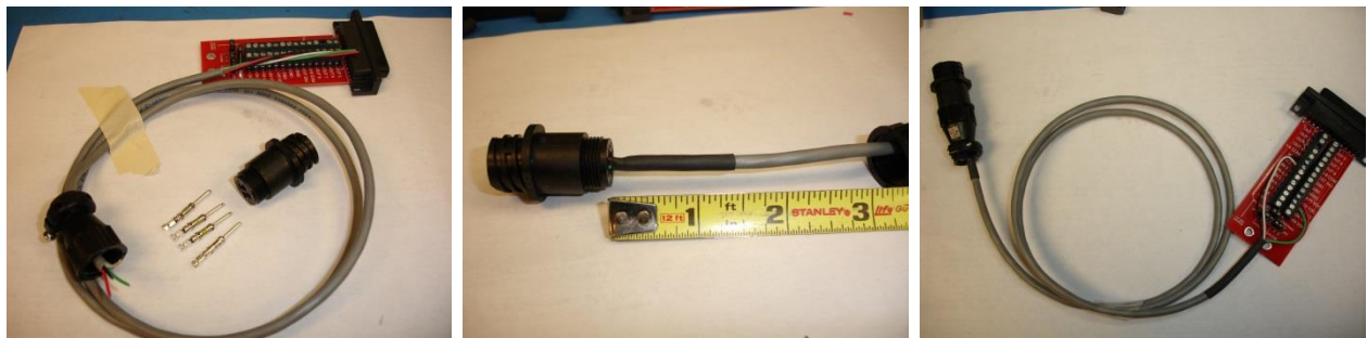
Figure 4. Terminating 4 Conductor Cable
