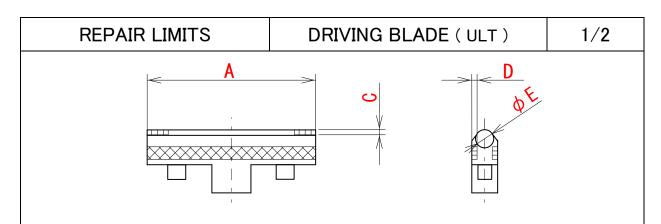
Note 1: Make sure that neither deformation nor damage is observed. Note 2: Make sure that no damage on contact surface is observed.
