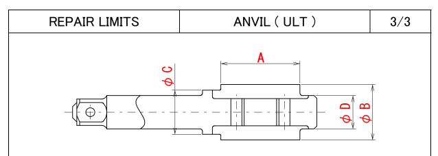
Note 1: Make sure that neither deformation nor damage is observed. Note 2: Make sure that no damage on contact surface is observed.
