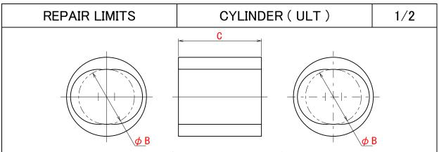
Note 1: Make sure that neither deformation nor damage is observed. Note 2: Mare sure that the inner surface is flat and smooth, not wavelike.
