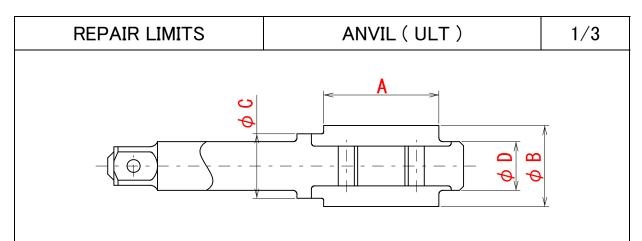
Note 1: Make sure that neither deformation nor damage is observed.
