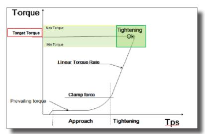
Enter the target torque, and the other fields are populated with default min/max torque.
