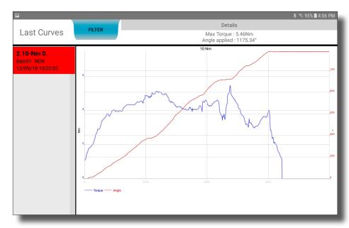
Torque is shown in blue, angle in red. To delete a curve, press your finger on the red curve for 2 seconds and select "Yes."
