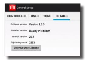
In the future, if you need to change to upgrade the software version (Start to Premium), click 5 times on the "Installed version" and enter the new key.
