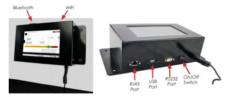
Ethernet RJ45 cables should employ a Ferrite if the cable length exceeds 10 meters to eliminate any external electrical interference within the local environment.
