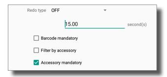
Filter by Accessory reduces the sequences shown on the menu "Select sequence" at the sequence link to the connected accessory. When an accessory is not connected, you will see the Screwdriver and 40 Nm sequence. When you attach the 200 Nm accessory, for example, you will see only the sequence where the extension 200 Nm is set up.
