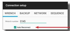
**Auto Reconnect:** When selected, the wrench will automatically reconnect to the controller when the operator changes the battery.
