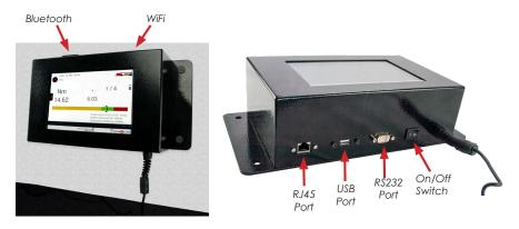
Ethernet RJ45 cables should employ a Ferrite if the cable length exceeds 10 meters to eliminate any external electrical interference within the local environment.
