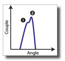
Screwdriver mode: Set angle target at 1°. Flexion mode: Set angle target to 2° or 3°.
