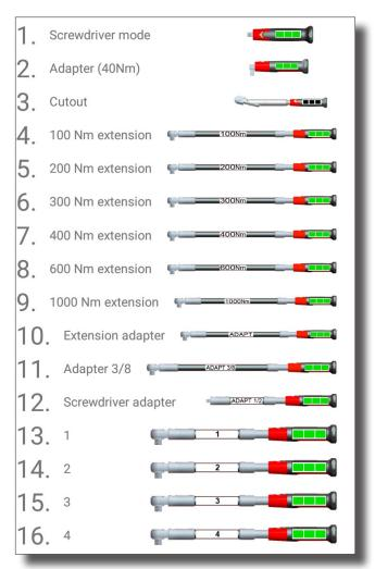
When choosing the accessory, take into account that accurate readings must be greater than 10% of the maximum torque for that accessory.
