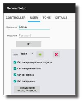
To require opearator sign-in prior to use of the wrench, activate the Tightening Permission function. To have the permission time out after X hours of use, enter that amount of time in the Control Frequency. The operator will be required to sign back in to the wrench once that time has elapsed.
