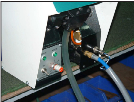
Correct Delivery Hose Installment
