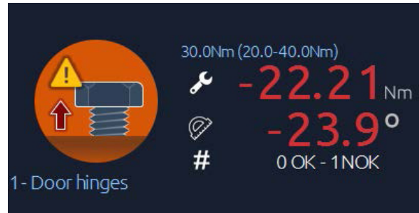
Figure 28 - Loosening Detected Screen
