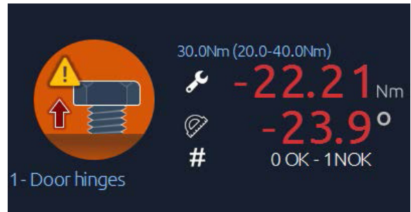
Figure 26 - Loosening detected screen
