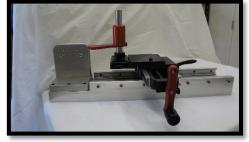
3: Attach transducer to angle bracket on main carriage. When inserting torque wrench into transducer, it is very important to adjust the wrench handle support so the torque wrench handle is level.
