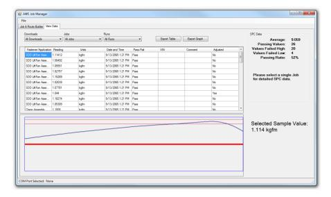
The trace file displays the data in a torque/time graph and allows the user to supersede the move-on reading selected by the wrench by visually discerning via the trace where the fastener started to rotate. When selecting a single job, the average, range, sigma, Cp and CpK values are listed.
