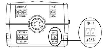
Connect between AM-45/AM-65 controller and the automation equipment via PCB: Connect A1 to K5, and connect H2 to H1. You can use the external controller to control the AM Controller. This is for automation ONLY.
