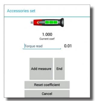
Apply a torque with the wrench on an external torque transducer and write the real torque in the field "Torque Read." Click on
