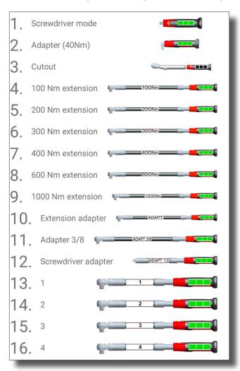
When choosing the accessory, take into account that accurate readings must be greater than 10% of the maximum torque for that accessory.
