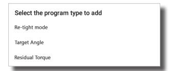
**Re-Tight:** Unscrew the screw from X° and retighten the screw back to the original position. The system records the disassembly torque and the torque when the screw returns to the same position.
