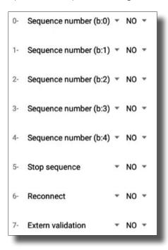
**Reconnect:** When this input is activated, the controller restarts the connecion with the wrench.
