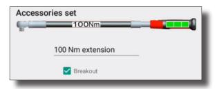
This function is need for the breakout (click type) extension and requires use of "Torque control & Angle monitoring" strategy.
