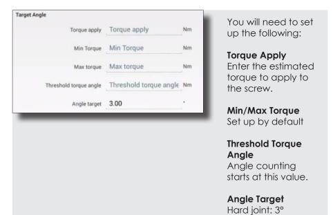
The breakout torque is measured when the angle target is reached. The angle target is set by default at 3°, but you can change it. The minimum value is 1°.
