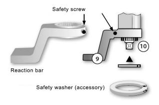
For reaction bars without safety lock, a safety washer is available as an accessory. This washer prevents a loosening of the reaction bar and can be pushed over the gear cogs and screwed tight.
