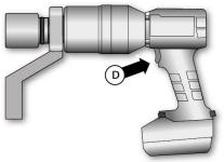
Switch on: Push and hold button (D). The electronic control system will ensure a soft start. Switch off: Release button (D).
