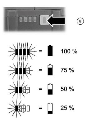
If one of the LEDs flashes, the battery pack is almost empty. The electronic circuitry protects the battery pack against damage due to complete discharge. Replace battery back on the power tool. Recharge battery pack.
