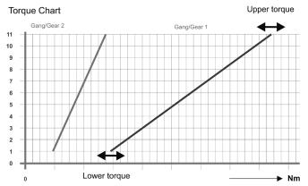
4) Reinstall battery pack after adjustment and check the settings using the SDMS. Repeat work steps until the required result is achieved. Document the torgue progression after completion.
