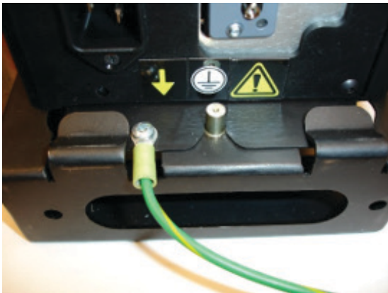
Figure 1 — Redundant Earth Ground Attachment
