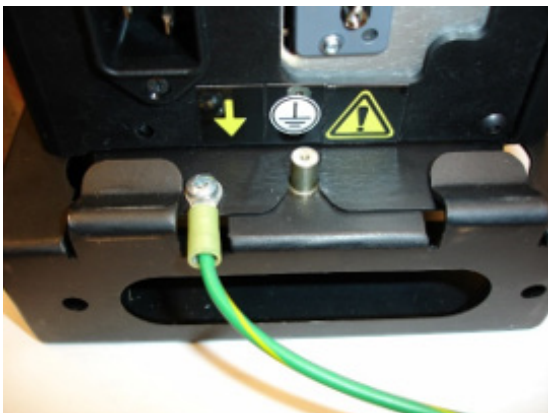
Figure 1 — Redundant Earth Ground Attachment
