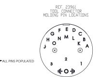
REAR VIEW ( PIN INSERTION SIDE OF MOLDING )
