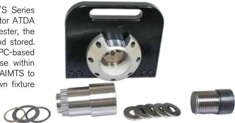
AIMTS-2000 Test stand for large impact tools
