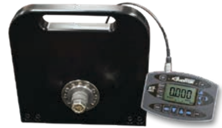
AIMTS-0500 Test stand for small impact tools. ATDA-DC Torque Data Analyzer sold separately.
