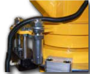
Parking brake and main rotation stops
