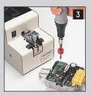
Bring screw to workpiece and fasten parts.
