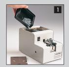
Load screws into the hopper. There is no side to load unit and no gates to limit capacity.
