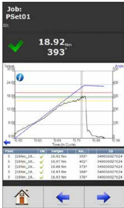
View curve results in real time or view stored results. As many as 20,000 curve results can be stored in memory.
