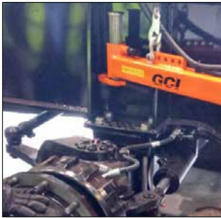
Rear Axle to Lower Section Target Torques = 265 nm, 800 nm
