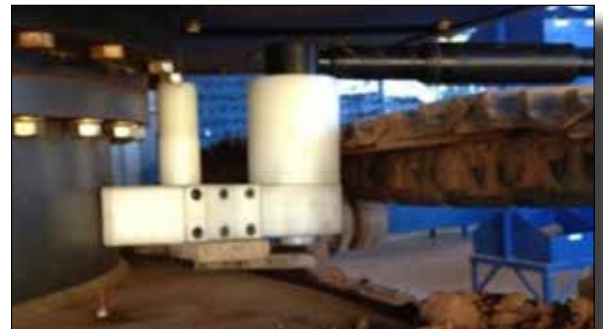
Final Assembly Tightening Car Swing Bearing
