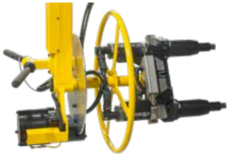
Two-Spindle System for Loader Wheels
