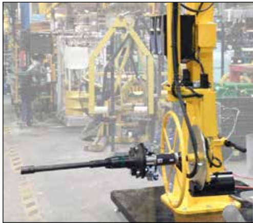
Two-Spindle System for Loader Wheels
